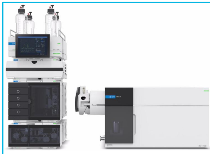
Figure 1. Infinity III 1290 and 6495D LC/TQ.
