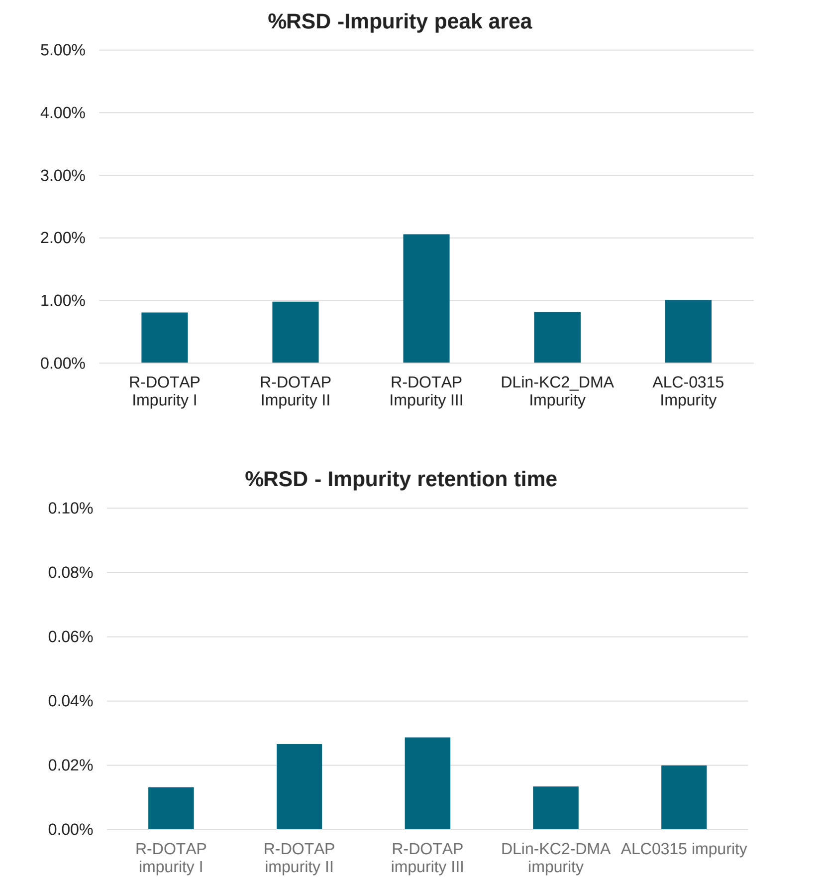
Figure 3: Impurity %RSD of peak area and retention time on CAD HP.
