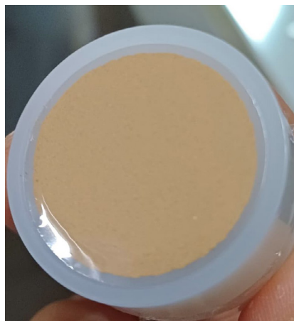
Figure 1. Picture of a coal fly ash sample prepared in as loose powder in liquid cup.
