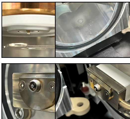
Fig. 3 Salt buildup in different components of the LC-MS/MS ion source after two direct seawater injections.
