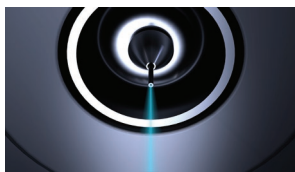
Fig. 4 CoreSpray Injection in the LCMS-8060RX
