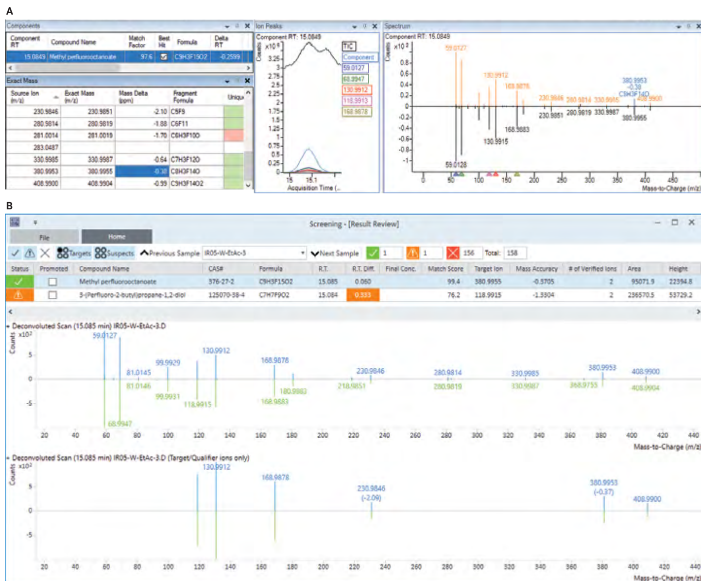
Figure 3. Example of PFAS (methyl perfluorooctanoate) identified in drinking water samples using PFAS PCDL in a nontarget approach using (A) Agilent MassHunter Unknowns Analysis software, and (B) a target GC/Q-TOF screening approach.
