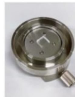
Underwater sample holder * Sample size \phi 20mm \times t3mm * Schematic
