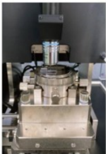
Standard sample holder ( \phi 50mm)
