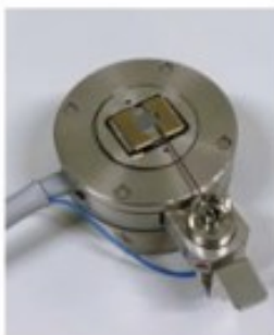
Heating holder * Sample size 10 \times 15 \times t3mm * Temperature range R.T \sim 250 ^{\circ} C (High load) R.T \sim 180 ^{\circ} C (Low load)
