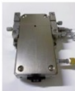
Cooling holder * Sample size 10 \times 10 \times t1mm * Temperature range -30 ^{\circ} C \sim 100 ^{\circ} C
