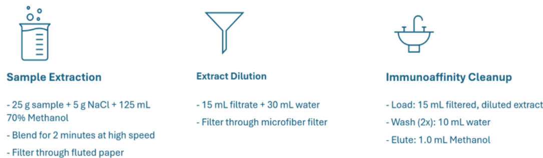
Figure 1: Representation of the sample preparation protocol for AOAC Official Method 991.31 Aflatoxins in Corn, Raw Peanuts, and Peanut Butter: Immunoaffinity Column (AflaTest) Method
