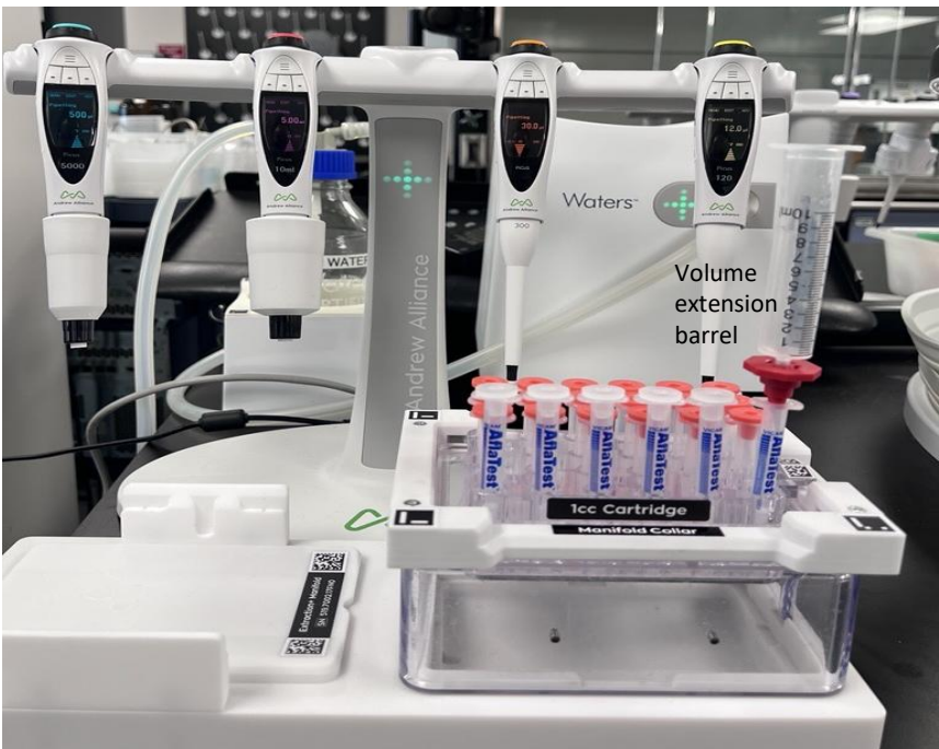
Figure 3: Compact setup allows cleanup of 24 samples at a time. A volume extension barrel is coupled to the cartridge to allow the entire sample to be loaded in a single step
