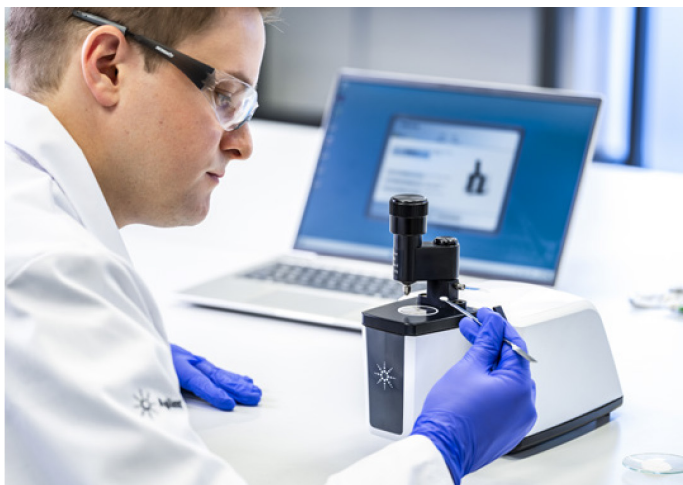
Figure 1. The Agilent Cary 635 FTIR spectrometer can be equipped with the right sampling modules to cover all analytical needs. The diamond ATR sampling module is ideal for the FTIR analysis of solids, liquids, gels, and powders.
