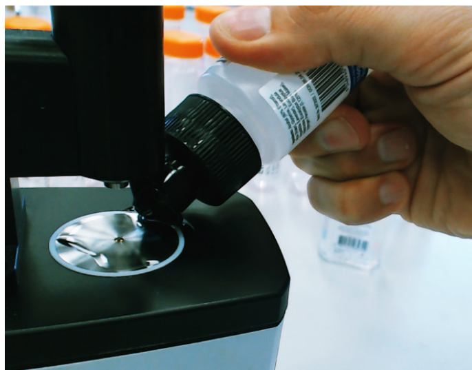
Figure 8. The neat hand sanitizer sample is placed onto the ATR accessory, fitted to the Agilent Cary 635 FTIR. The Agilent MicroLab software uses picture-guided workflows to help users follow each step of the measurement including cleaning and sampling.
