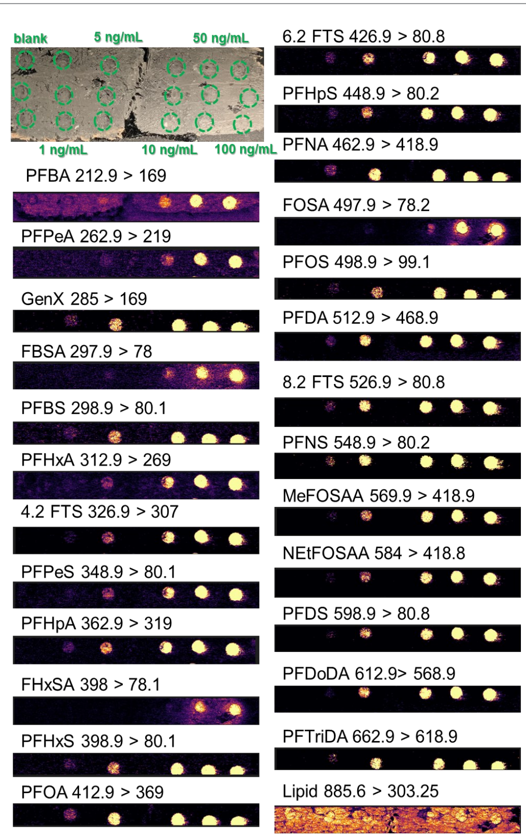
Figure 1. Ion images of PFAS mix dilution series spotted on porcine liver tissue section from 1 ng/mL up to 100 ng/mL acquired using DES XS on the Xevo TQ Absolute MS in targeted MRM acquisition mode .
